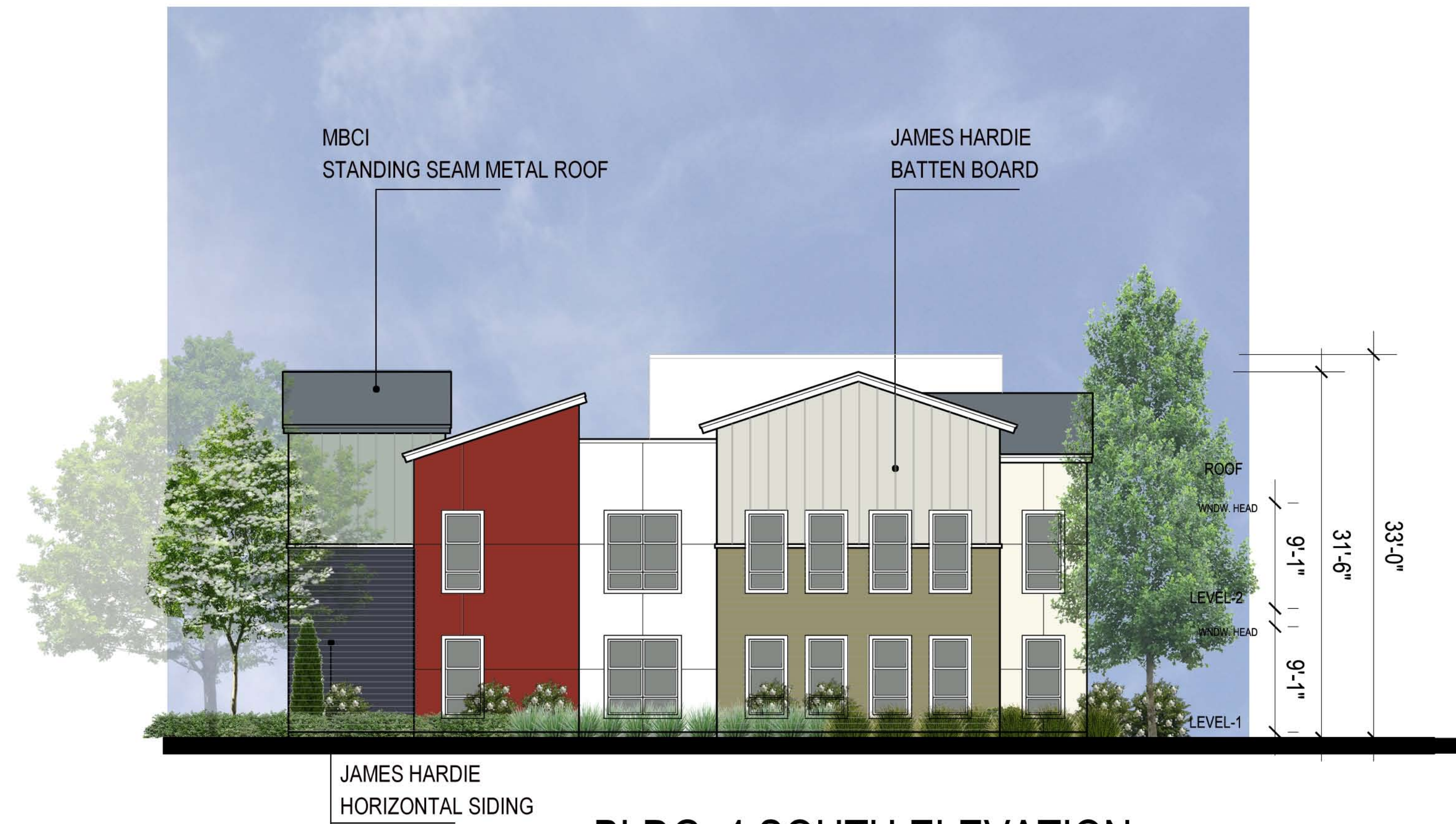
BLDG. 4 SOUTH ELEVATION
