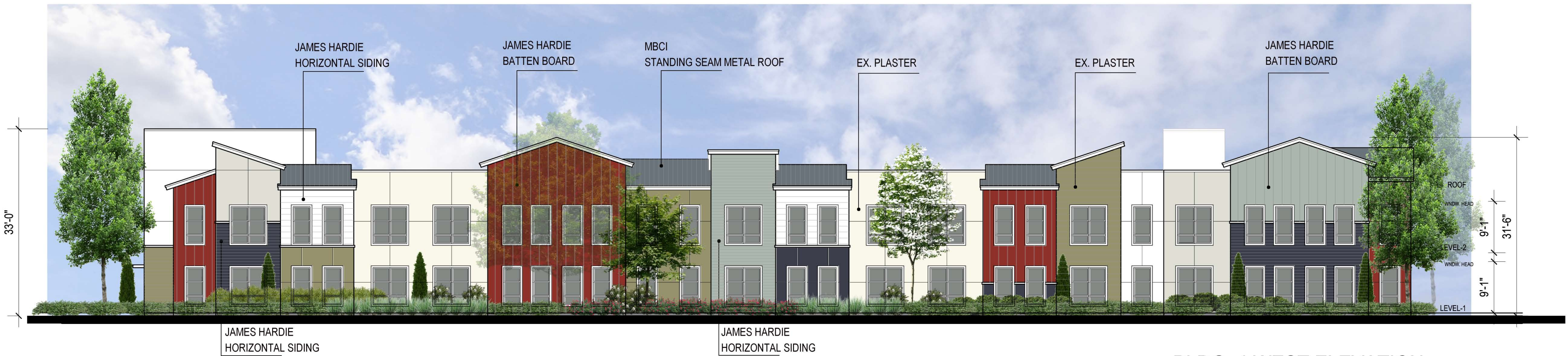
BLDG. 4 WEST ELEVATION
